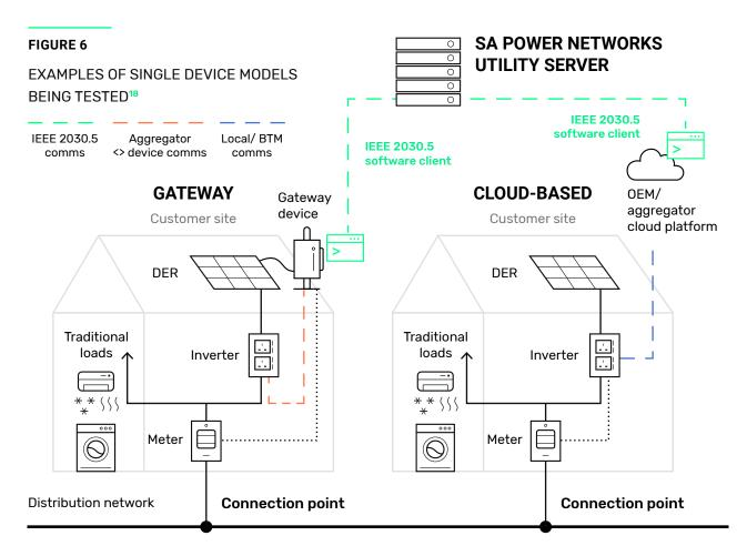
Although it is the smart inverter receiving and acting on the DOE, the power flows of the entire site still need to be considered.
